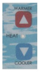
To enter the programming mode, press and hold both the **WARMER** and **COOLER** buttons at the same time for **3 seconds**. The display will indicate the filter mode with a code (F1 indicates Filter Mode 1, etc.).
