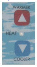
**Temperature Buttons** - You control the water temperature with the **Warmer** (up arrow) and **Cooler** (down arrow) Buttons. Each time you press a button, the Set Temperature changes by one degree. For your safety, the temperature can be set no higher than  $104\,^{\circ}$  F ( $40^{\circ}$  C).
