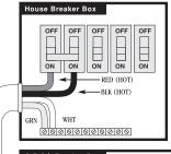
Note: The white neutral wire from the back of the GFCI MUST be connected to an incoming line neutral. The internal mechanism of the GFCI requires this neutral connection. The GFCI will not work without it.
