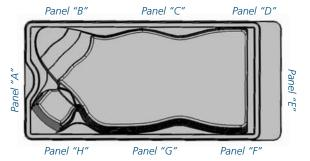
**NOTE:** The above drawing illustrates panel placement on the H2X. The CrossTrainer is labeled the same. **WARNING:** Do Not Remove Access Panels Without Turning Off Power To The Swim Spa.
