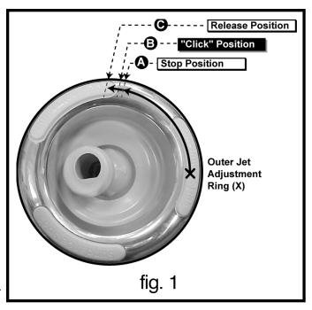
are overtorquing the jet internal between positions (A-B), however, additional force is necessary at position (A) to unlatch its retaining mechanism from the wall fitting.
