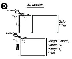
Rinse debris from all filter pleats using a garden hose and high-pressure nozzle. Start at top and work downward to face. Repeat process until all filter pleats are clean.
