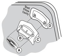
2. Use a standard screwdriver to loosen and remove mounting bolts (B) from pillow base, then remove pillow base from shell cavity (D).
