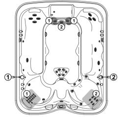
Pump 1 Powers All Unmarked Jets Massage Selector #1 Controls Pump 2 Massage Selector #2 Controls Pump 3
