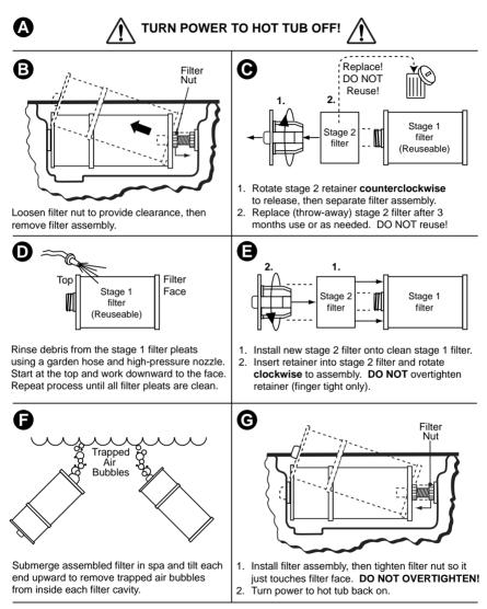
Periodically, the stage 1 filter will need a more thorough cleaning to remove imbedded oils and minerals. For this, we suggest cleaning as illustrated above (step D), followed by soaking the filter overnight in a plastic container filled with a solution of water and a specially formulated filter cleanser available from your Sundance dealer.
