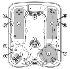
**8.5 Jets 1:** The sensor pad labeled **JETS 1** controls the 2-speed pump #1. Press once for low speed. Press a second time for high speed. Press a third time to turn off.
