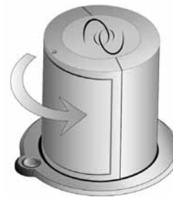
Rotate speaker counter-clockwise to return to the initial raised position in order to lower speaker.
