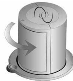
Rotate speaker to return to the initial raised position in order to lower speaker.
