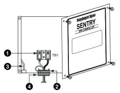
Figure-D Terminal Block 240V **Wire Connection**
