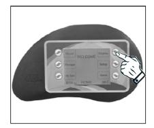
The first step is to touch the button next to the "**DISPLAY**" box. This will open a screen that allows you to brighten or darken the display.
