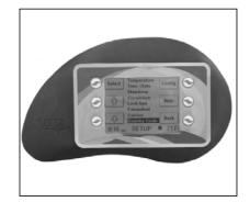
Use "**UP**" and "**DOWN**" arrows to cycle past the selections. Use the "**SELECT**" key to choose your selection then adjust accordingly. Press "**BACK**" to return to main screen.
