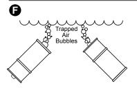
Submerge assembled filter in spa and tilt each end upward to remove trapped air bubbles from inside each filter cavity.
