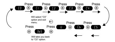
1. After the last cycle, "C6," the LED screen will display "U" or "O3." If the LED screen is displaying "U" then pressing the Jets pump 1 will change the sanitizing system from "U" to "O3" and exit the programming menu. If the LED screen is displaying "O3" then pressing the Jets pump 1 will change the sanitizing system from "O3" to "U" and exit the programming menu. You will see one of the two configurations below:
