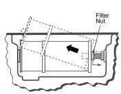
Loosen filter nut to provide clearance, then remove filter assembly.
