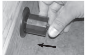
6. Thread the cap back on the push the internal back into the housing until it snaps into place.
