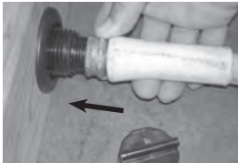
5. To disconnect the hose, push the hose inward approx. 1/2" to shut the water flow off. Unthread the hose.
