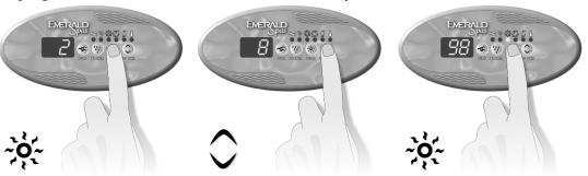
Press and hold Light key for 5 seconds. The display will show a value that represents the filter cycle duration in hours. Use Up or Down arrow key to change setting.
