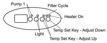
**Default System Operation:** When power is applied, or there is a temporary loss of power, the system will initiate its default programming. The filter cycle will begin24-hours after the system has been powered up. The filtration cycle will be active for 1-hour and will repeat every 12-hours. The temperature will be maintained at 95° F. (Default setting can change) w/out notice
