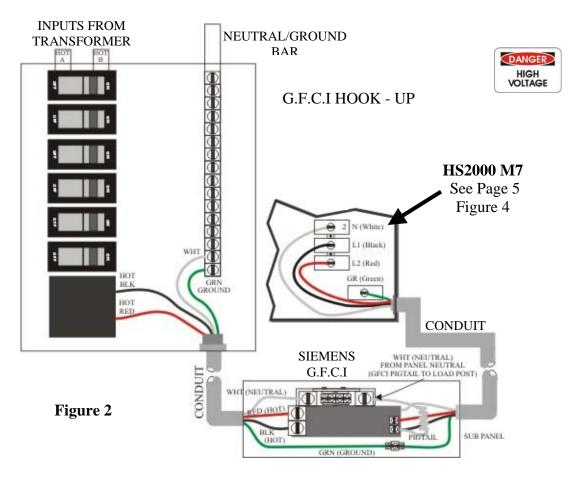
An illustration showing the proper electrical connections for 240 volt service has been provided for you. (Figure 2) Be sure to follow these and all other instructions carefully. Be sure that all connections are tight before switching on the circuit breaker.
