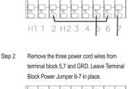
Remove the Terminal Block Power Jumper
