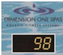
**The Display Window** shows the current water temperature, except when you are adjusting the temperature using the Warmer and Cooler buttons. Then it shows your desired **Set Temperature**. Five seconds after you finish setting the desired temperature, the Display Window reverts to showing the current temperature.
