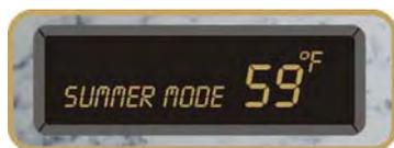
To initiate **SUMMER MODE**, use the Down Button to set the temperature below 59° F (@15°C). **SUMMER MODE** will appear in the Display Window. In this mode the pump will run the filter cycle until the water reaches 107°F (@41° C) before turning off. It will remain off until the water temperature falls to 102° F (@38° C) at which point the pump turns on again.
