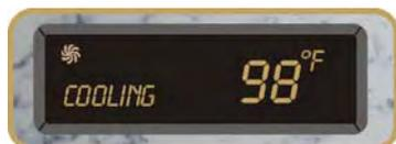
When “**COOLING**” appears beside the water temperature in the Display Window, the water temperature has reached 2° F ( $\cong 1^{\circ}$  C) above the set temperature. The circulation pump and ozone generator will turn off to allow the water to cool back to the set temperature. This is a normal hot tub function. No corrective action is necessary.
