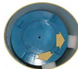
7. Remove either of the two filters from the pool side of the system. (If you have the Dual-Temp model with separate built-in spa, also remove the filter from the spa side). Fill the system with water by placing a garden hose in the empty filter canister. (If you need more details on how to remove the filters, see the Filter Cleaning section later in this manual.)
