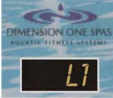
**L1 - PUMP LOCKOUT** – You can use the **L1** mode to prevent any pumps from accidentally running while you're cleaning the filters or doing any type of non-electrical servicing on your System.
