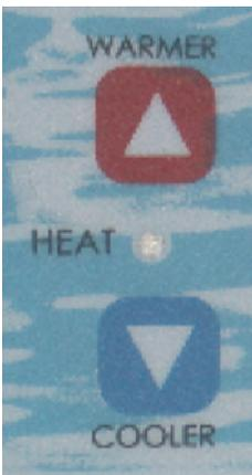
To enter the programming mode, press and hold both the **WARMER** and **COOLER** buttons at the same time for **3 seconds**. The display will indicate the filter mode with a code (F1 indicates Filter Mode 1, etc.).
