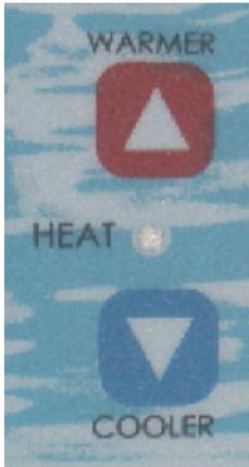
**Temperature Buttons** - You control the water temperature with the **Warmer** (up arrow) and **Cooler** (down arrow) Buttons. Each time you press a button, the Set Temperature changes by one degree. For your safety, the temperature can be set no higher than 104 ° F (40° C).
