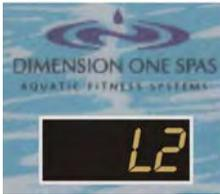
**L2 - PANEL LOCKOUT** – The L2 Lockout function prevents unauthorized use of your system by disabling the Control Panel.
