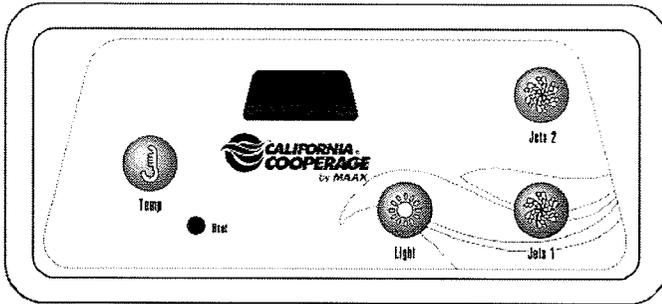
The California Cooperage® Model 137 Control System is used on Spa Model 107.
