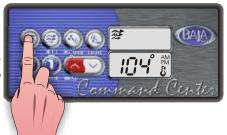
**Jet 2 Key:** Press this key once to turn Pump 2 onto High speed, a second press will turn the pump off. A built-in timer will shut the pump off after 20 minutes of operation unless done so manually. The Pump 2 Icon will appear in the upper LCD window while the pump is running in High speed (WhiteWater™ Series Only).
