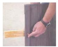
Attach coupling blocks to one end of side panel with toggle bolts and tool supplied with cabinet.
