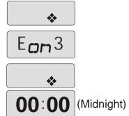
**Economy Duration 3: ("Edu3")** appears in the display. To adjust, **(1)** press the Enter (Light) key. Use the Warmer/Cooler keys to adjust from OFF (always off) to 24 (always on). **(2)** Press the Program key to confirm the new setting and exit to the Time/Temperature display. **FACTORY SET OFF**
