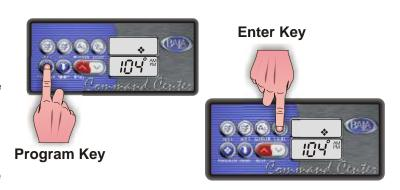
**Time of Day:** This is the first parameter and will automatically appear with the hour flashing. To adjust, (1) press the **Enter (Light) key**, use the Temp. Set keys to adjust the hour from 00: to 11:. (2) Press the **Program key** then **Enter (Light) key** to adjust minutes, use the Temp. Set keys to adjust the minutes from :00 to :59. (3) Press the **Program key** to confirm the new setting and move to the next parameter to be programmed.
