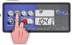
Blower Key: Press this key once to turn the Blower onto High speed, a second press will turn the Blower onto Low speed, a third press will turn the Blower off. A built-in timer will shut the blower off after 20 minutes of operation unless done so manually. The Blower Icon will appear while the blower is running in High speed and flash while it is in Low speed.
