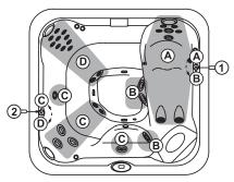
Massage Selector #1 Controls Pump 1 Massage Selector #2 Controls Pump 2 Foot and Side Wall Jets E Powered by Pump 3
