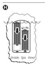
Place each cartridge back into skimmer well\*, then rotate each cartridge handle clockwise to thread back into wall fitting. DO NOT OVERTIGHTEN!
