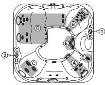
Massage Selector #1 Controls Pump 1 Massage Selector #2 Controls Pump 2 Foot and Side Wall Jets E Powered by Pump 3
