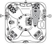
Massage Selector #1 Controls Pump 1 Massage Selector #2 Controls Pump 2
