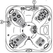
Massage Selector #1 Controls Pump 1 Massage Selector #2 Controls Pump 2
