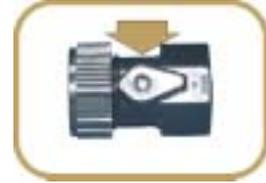
4. Close the valve on the side of the hose bib and screw it onto the end of the hose bib. Check to ensure the cap on the hose bib is secure to avoid leaks when you add water to the spa.
