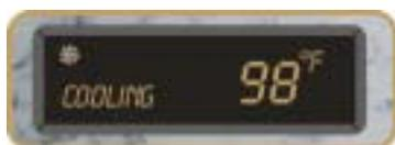
When “**COOLING**” and the water temperature are displayed on the Digital Display Window, the water temperature has reached 2° F ( $\cong$ 1° C) above the set temperature. The circulation pump and ozone generator will turn off to allow the water to cool back to the set temperature. This is a normal hot tub function. No corrective action is necessary.
