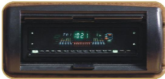
The optional Sonic Immersion System provides a superior fidelity and low distortion stereo system featuring patented planar magnetic speaker technology (1/4" thick) that generates unparalleled sound quality – even in the harshest environmental conditions.
