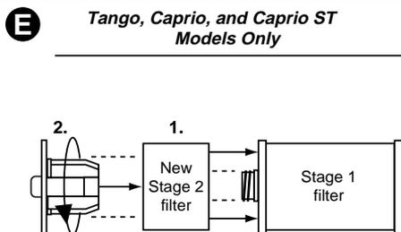
1. Install new stage 2 filter onto clean stage 1 filter.
