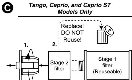
1. Rotate stage 2 retainer **counterclockwise** to release, then separate filter assembly.
