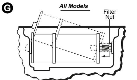
1. Install filter assembly, then tighten filter nut so it just touches filter face. **DO NOT OVERTIGHTEN!**
