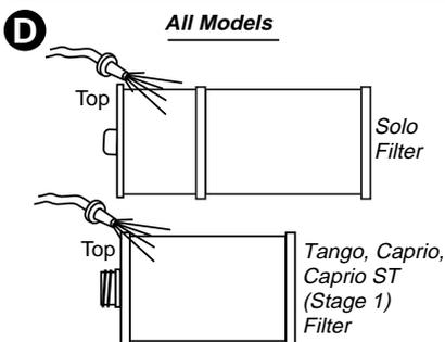
Rinse debris from all filter pleats using a garden hose and high-pressure nozzle. Start at top and work downward to face. Repeat process until all filter pleats are clean.
