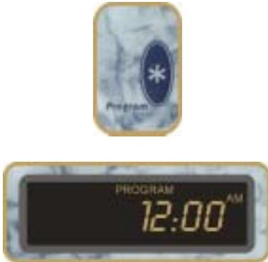
**Program Button:** The **PROGRAM Button** is used to set several different functions including:
