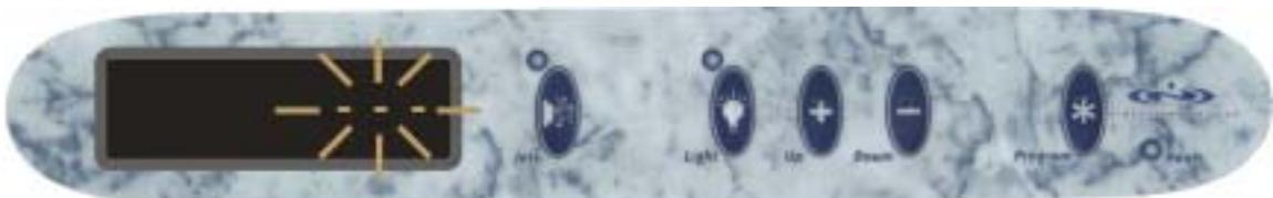
13. Push the **JETS 1 Button** twice to turn the pump to high speed. Let the system run for 30 to 45 seconds to prime the pump. Then push the button again to shut the pump off. Repeat the process with the other pump using the **JETS 2 Button**.
