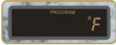
**Program the Temperature Unit** by pressing the **PROGRAM Button** a 5<sup>th</sup> time. The current Temperature Unit will be visible in the Digital Display Window.
