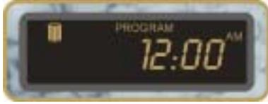
**Program the Filter Cycle Start Time** by pressing the **PROGRAM Button** a 2<sup>nd</sup> time. Whenever you are programming a filtration setting, the **FILTER Icon** will be displayed next to the word **PROGRAM** in the Digital Display Window.
