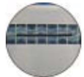
12. Once the spa is full, turn on the circuit breaker (not supplied by Dimension One Spas). Flashing dashed lines will appear for 30 seconds on the Digital Display Window followed by the current water temperature (flashing). The Top Side Control, shown below, will vary depending on your model of spa.
