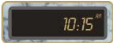
**Dimension One Spas ICON (Logo):** The time of day can be viewed by pushing the **Dimension One Spas ICON Logo Button** on the far right of the control. If no other button is pushed within 5 seconds, the display will revert to the spa water temperature reading.
