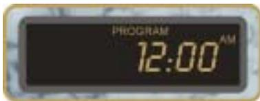
**Program the Clock** by pressing the **PROGRAM Button** and holding it for about 5 seconds. The Digital Display Window will display the word PROGRAM and a digital clock with the HOUR setting flashing.
