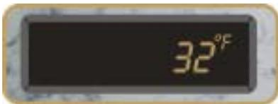
**DO NOT ENTER THE WATER** if you see a temperature reading of 32° F ( $\cong$ 0° C) or 136° F ( $\cong$ 57.8° C) without first checking the actual water temperature with a separate thermometer. The system has detected a Temperature Probe Failure and the water may be too hot, or too cold, to safely use.
