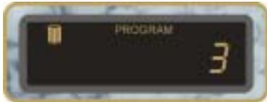
**Program the Number of Filter Cycles** by pressing the **PROGRAM Button** a 4<sup>th</sup> time. Whenever you are programming a filtration setting, the **FILTER Icon** will be displayed next to the word **PROGRAM** in the Digital Display Window.
