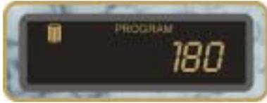
**Program the Filter Cycle Duration** by pressing the **PROGRAM Button** a 3<sup>rd</sup> time. Whenever you are programming a filtration setting, the **FILTER Icon** will be displayed next to the word **PROGRAM** in the Digital Display Window.
