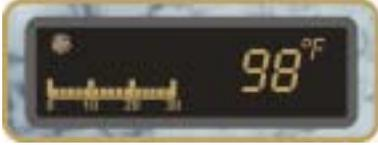
A built-in timer will automatically shut the pump off after 30 minutes of operation unless you turn it off manually. When the pump is first turned on, a small scale will be displayed in the lower left corner of the Digital Display Window.
