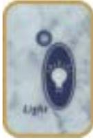
**Light Button:** Push the **LIGHT Button** once to activate the brightest setting. A second push will activate the medium setting, and a third push will activate the dimmest setting. Push the **LIGHT Button** a fourth time to turn the light off. When the spa light is ON, the Light Indicator LED will be lit. The light will automatically turn off after one hour. A Light Icon will also display in the upper left corner of the Digital Display Window whenever the light is on.
