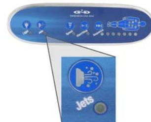
17. Then push the **Jets Button** on the other Dynamic Massage Sequencer to prime its pump. Let it run for 10 to 15 seconds, then press the button again to shut the pump off.
