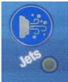
The Jets button on the Dynamic Massage Sequencer turns the jet pump associated with the Sequencer on or off. The same spa jet pump jet may be turned on or off using the button on the **d r i v e** Control Panel.
