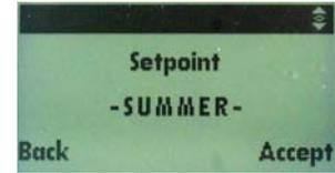
To enter Summer Mode, adjust the set point to the lowest possible temperature, 59°F (15°C), and continue to hold the down arrow on the 5-Key Context Keypad. The temperature value will be replaced by "Summer."
