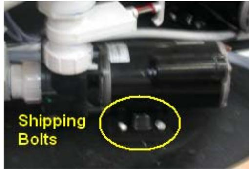
8. Next, look at the two circulation pumps located at the bottom of the main equipment compartment. Check the hose clamp fitting where the plumbing attaches to the pumps and make sure they are tight.
