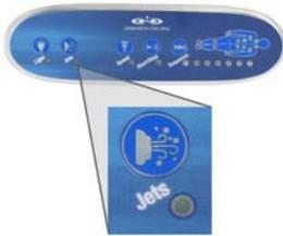
Push the Jets button to turn on the jet pump.
