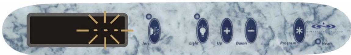
13. Push the **JETS Button** twice (use the **JETS 1** Button on multi-pump spas) on North American 60Hz models to turn the pump on to high speed. (Push it once on European 50Hz models). Let the system run for 30 to 45 seconds to prime the pump. Then push the button again to shut the pump off. If your spa has two jet pumps, repeat the process using the **JETS 2 Button**. Replace the bleeders once the pumps are running properly.
