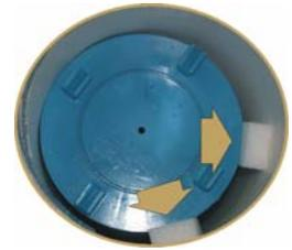
10. If your spa has two filters, remove the UltraPure™ filter (see photo to the left) and fill the spa with a hose in that canister. Otherwise, remove the single filter and fill the spa through that canister. (You can see Filter Cleaning instructions in this manual to learn more about removing filters).
