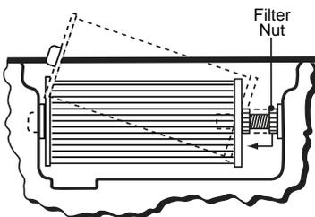
1. Install filter, then tighten filter nut so it just touches filter face. **DO NOT OVERTIGHTEN!**
