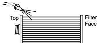
Rinse debris from filter pleats using a garden hose and high-pressure nozzle. Start at the top and work downward to the face. Repeat process until all filter pleats are clean.
