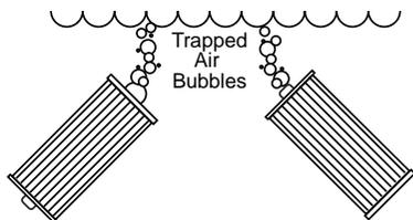
Submerge filter in spa and tilt each end upward to remove trapped air bubbles from inside each filter cavity.
