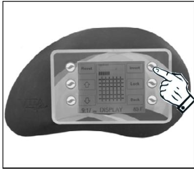
Press the **"INVERT"** button and the screen will clear and reset itself. As with many computer screens, the change in display may take up to 30 seconds to be completed.
