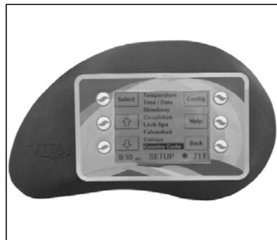
Use **"UP"** and **"DOWN"** arrows to cycle past the selections. Use the **"SELECT"** key to choose your selection then adjust accordingly. Press **"BACK"** to return to main screen.
