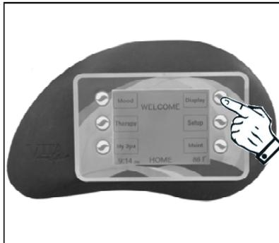
The first step is to touch the button next to the **"DISPLAY"** box. This will open a screen that allows you to brighten or darken the display.
