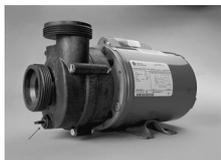
Screw pump plug into face of pump.
