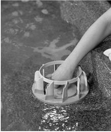
Turn filter cartridge counterclockwise to unscrew.
