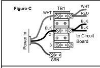
North American Convertible Models: 120/240 VAC, 3-Wire Connection 60 Hz North American Convertible Models: 120/240 VAC, 4-Wire Connection 60 Hz
