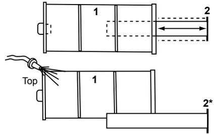
Lightly rise filter insert (2) and place in clean location. \*DO NOT use chemical cleaners or high-pressure nozzle on insert (2) or it may be damaged, come apart or allow impurities to re-enter the water, increasing the risk of contracting a waterborne illness (e.g. an infection bacteria or virus) and/or respiratory ailments.
