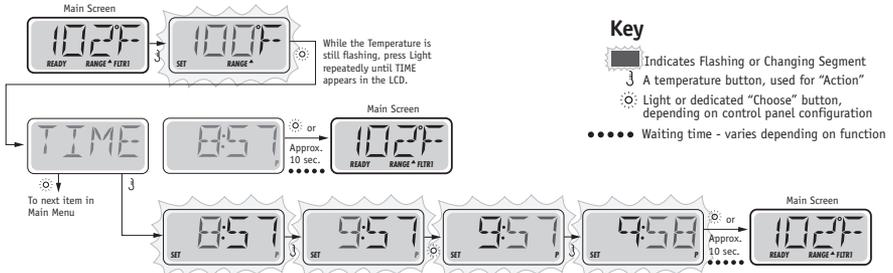
**NOTE:** If power is interrupted to the system, Time-of-Day will need to be reset.
