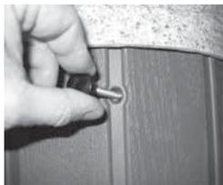
2.) Remove front side panel (this is the side where the main topside control panel is located) so the electrical service can be hooked up to the spa system pack. The panels can be taken off by first removing the three black thumb screws located on each corner. On the center panel there are four #2 Phillips screws that are covered with a colored snap cap. Remove the caps to access the screws for removal.
