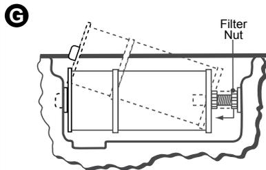
1. Install filter assembly, then tighten filter nut so it just touches filter face. **DO NOT OVERTIGHTEN!**
