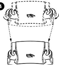
Gently pull outward on pillow to release mounting stud from receptacle on spa shell.
