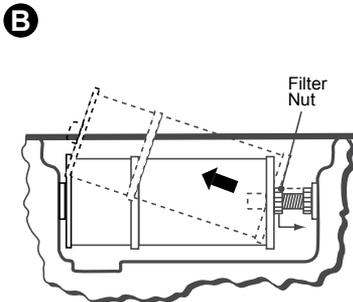
Loosen filter nut to provide clearance, then remove filter assembly.
