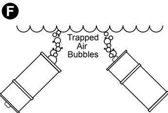
Submerge assembled filter in spa and tilt each end upward to remove trapped air bubbles from inside each filter cavity.
