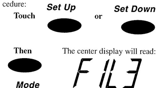
Adjust the cycle duration by pushing the set up or set down pad. Each press of the pad will display which filtration cycle you have chosen:
