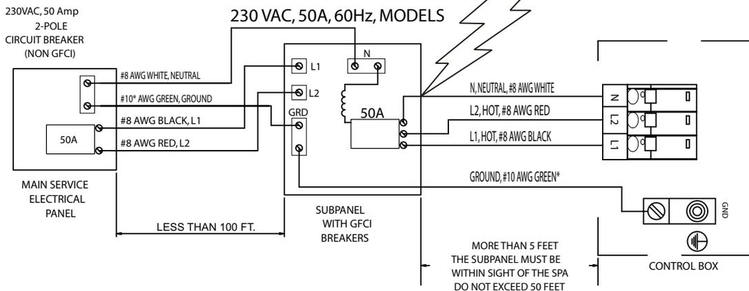
\*ALL CANADIAN SPA MODELS USE #8 AWG GREEN, GROUND. THESE SPAS ARE INTENDED FOR USE WITH GFCI SUBPANEL.
