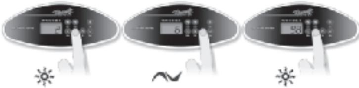
Press and hold Filter key until the display shows "x", representing the currently set filter cycle duration in hours.
